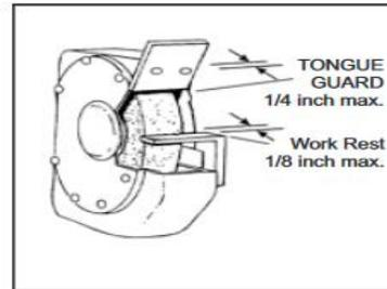
The bench grinder (sometimes called an offhand or pedestal grinder) is one of the most common pieces of equipment found in a shop setting. It has a multitude of uses, but can also cause serious injuries if not operated correctly.
